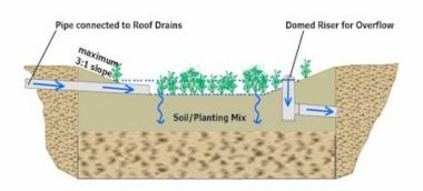
A Rain Garden (also called Bioretention) is an excavated shallow surface depression planted with specially selected native vegetation to treat and capture runoff.
