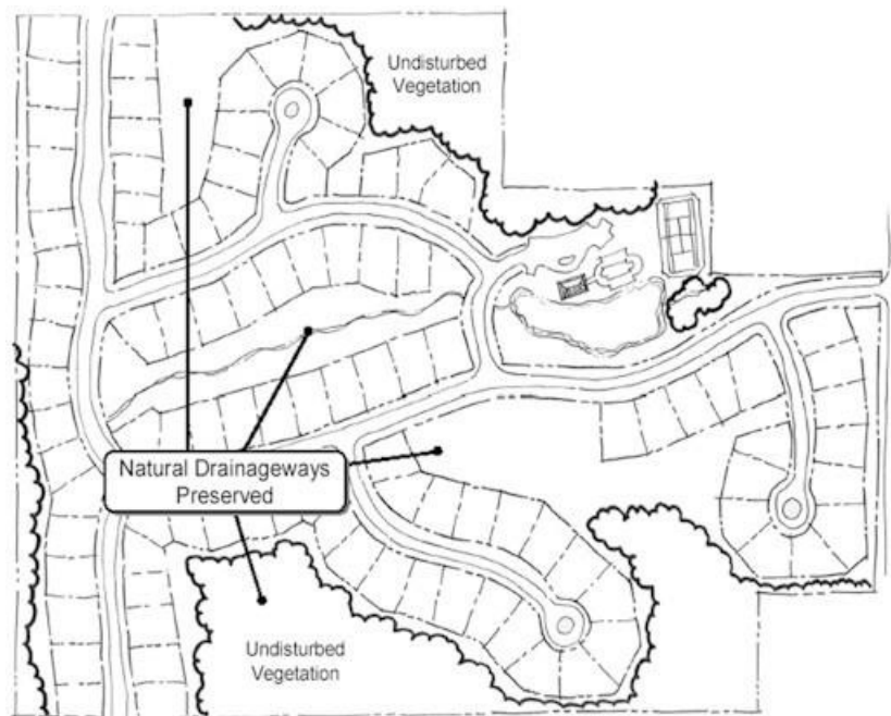
Figure 5.3-1 Protect natural drainage features
