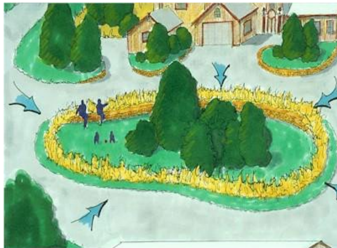
Figure 5.3-6 Natural surface depressions can temporarily store stormwater.
